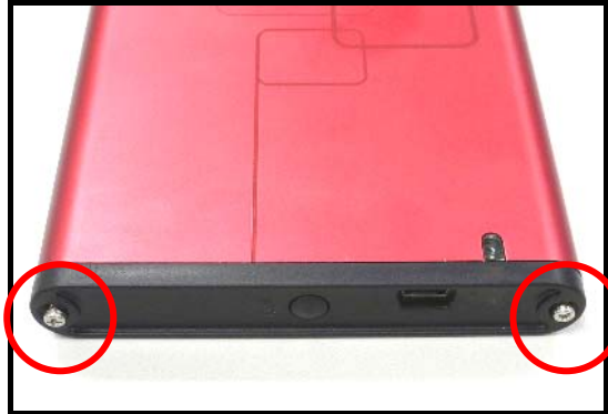
Figure 2. Remove the screws from the top cover
