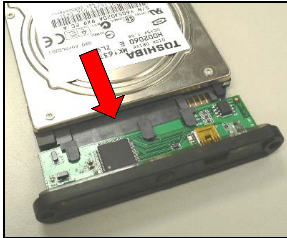
Figure 4. Connect the hard drive to the IDE/SATA adapter
